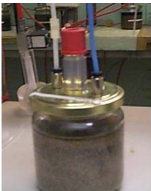
Fig. 3.7: Glass jars with modified twist off lid with an in and out flow connection to the aeration and GC system and septum closed cylinder for water addition.
