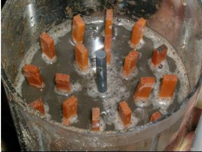
Fig. 3.6: Arrangement of wood samples in the upper layer of a microcosm (a plastic stick was used in the middle of the MC as placeholder for the later added decayed wood)
