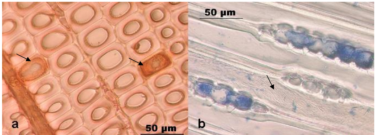
Fig. 6.9a, b: Examples of bacterial decay (arrowed) most often observed in the second MC experiment II a) transverse section b) longitudinal section, (from Kretschmar et al. 2007a)
