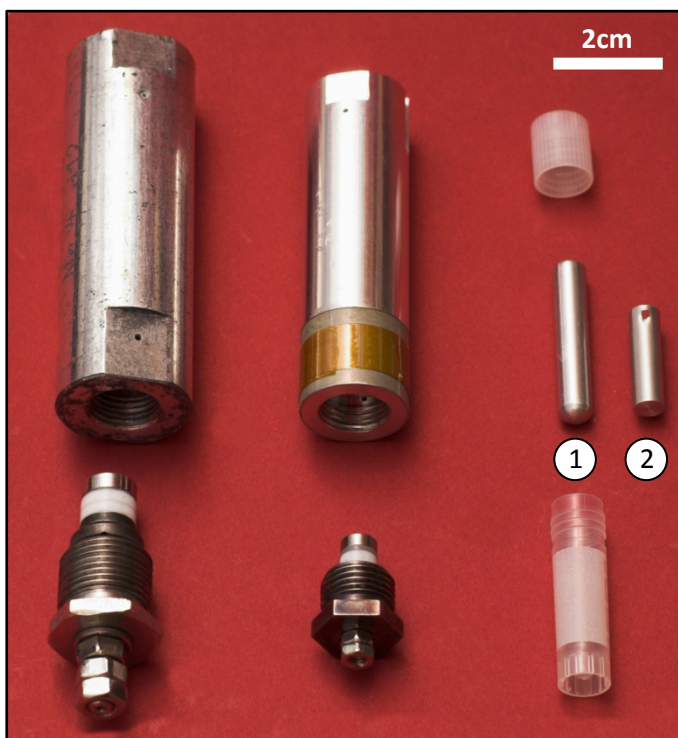
Fig. 66) Experimental cells with Bridgman seals used in pVT (left most) and neutron diffraction (middle one with Cd plating) experiments. Aluminum vials (1) like the one from the right hand side were filled with a sample and inserted into the cells or mounted to the cold head on the BW5. For a few ex-situ X-ray diffraction experiments, some samples were transferred to smaller vials (2) and slipped into vials (1) with different samples.
