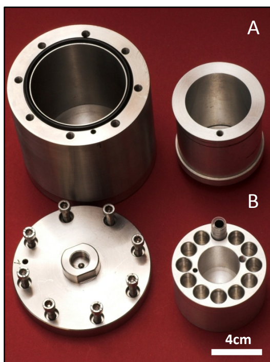
Fig. 68) Experimental cell used to produce large volumes of clathrates for decomposition runs. Hydrate cores for powders (4.2.1) were prepared in the insert A. Consolidated samples were formed directly in the aluminum vials (insert B).
