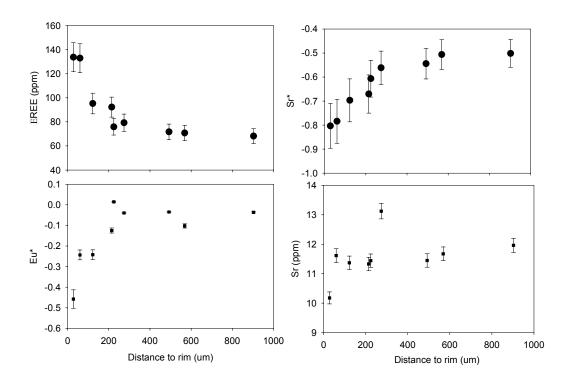
Fig. 4.8 Compositional profile of clinopyroxene in sample 24. EREE = total concentration of REEs, Eu\* (Eu anomaly) = $Eu_N/[(Sm)_N(Gd)_N]^{1/2}$  -1, Sr\* (Sr anomaly) =  $Sr_N/[(Ce)_N(Nd)_N]^{1/2}$ -1 (Wood et al., 1979), where subscript N means chondrite normalization.
