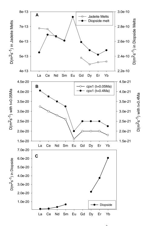
Fig. 6.13 Comparison of REE diffusion coefficients (D,  $m^2s-1$ ) in different media: (A) REE diffusion data in jadeite and diopside melt, form experimental studies at 7.5 kbar-1400°C and 10kbar-1590°C respectively (Nakamura and Kushiro, 1998); (B) REE diffusion data in clinopyroxene, from this study. (C) REE diffusion data in high-Ca diopside, calculated for 1200°C and 1 atm with diffusion parameters given by Van Orman and Grove, 2001.
