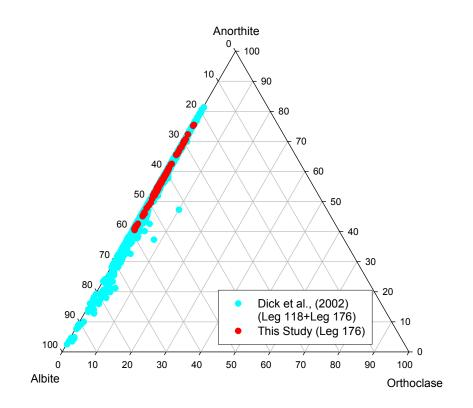
Fig. 4.1 Feldspar ternary plot of plagioclase from Hole 735B gabbros. All compositions define a very tight trend close to the anorthite-albite join, with anorthite contents ranging from  $An_{40}$  to  $An_{80}$ . Compared with the whole data set, plagioclase with anorthite content lower than  $An_{40}$  is absent in this study, which is believed to reflect the scarcity of felsic veins in the lower part of this gabbro block.
