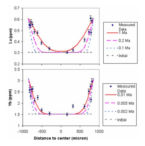
Fig. 6.9 Diffusion modeling of La and Yb in CPX1. Measured results are given in Table 4.3, diffusion rates are calculated with the diffusion parameters given by Van Orman et al. (2001) at a temperature of  $1200^{\circ}$ C.
