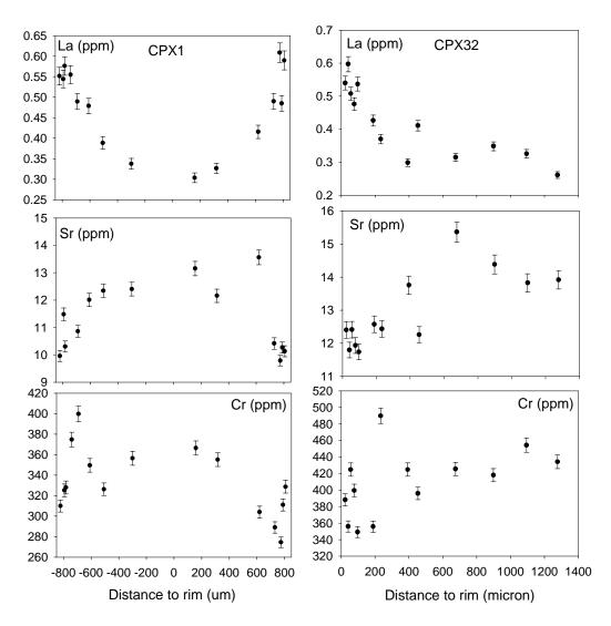
Fig. 4.10 Trace element zoning profiles acquired by *in-situ* ion probe analysis in CPX 1 and CPX 32. Sr and Cr show larger space variations, however most data points are still following along continually changed zoning profiles.
