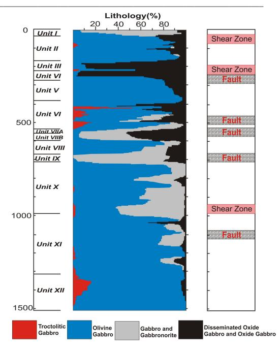
Fig. 2.2 Summary of lithostratigraphy and deformation of Hole 735B.
