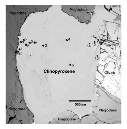
Fig. 6.5 Reflected light photograph of analyzed clinopyroxene grain in sample 1 (cpx 1), which is surrounded by plagioclase and olivine. Analysis numbers are given beside ion probe pits (black dot). Analysis run across the whole grain with most pits in the outmost ~400 microns rim area to define the zoning profile of trace element, beyond that distance the concentrations of measured trace elements become constant in the core area (see text for discussions).
