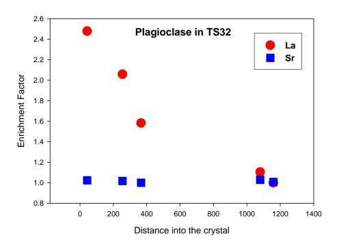
Fig. 4.3 Compositional variation of plagioclase in TS32 (TS-Thick Section) from Hole 735B gabbros. Enrichment factor=  $C/C_0$ , where C is the measured concentration at any position,  $C_0$  is the concentration at core position. Compared with the significant enrichment of La to the rim, Sr has a nearly constant content throughout the crystal.
