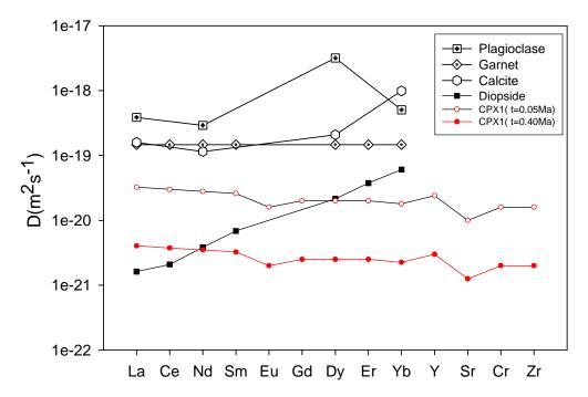
Fig. 6.11 Trace element diffusion coefficients in various minerals. Sources of data: Diopside – Van Orman and Grove, 2001; Garnet – Van Orman et al., 2002; Plagioclase – Cherniak, 2002; Calcite – Cherniak, 1998. For comparison diffusion coefficients in diopside, garnet, calcite, and plagioclase are the calculated at the same temperature of  $1200^{\circ}$ C by Arrhenius equation with diffusion parameters given in the related literature.
