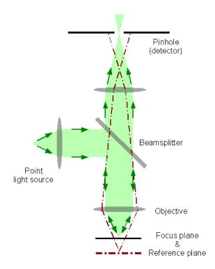
Fig. D.3: Principal setup of a Confocal microscope
