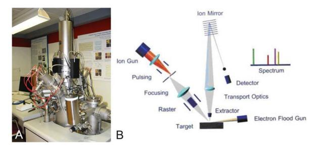
Fig. 1.7 (A) ToF-SIMS IV Instrument used in this study at the SP Technical Research Institute of Sweden, Borås, and (B) scheme of the ToF-SIMS principle, image courtesy of ION-TOF GmbH, Münster).
