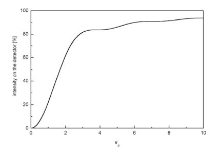
Fig. D.4: Collection efficiency as a function of the pinhole size normalized to the total power in the image plane
