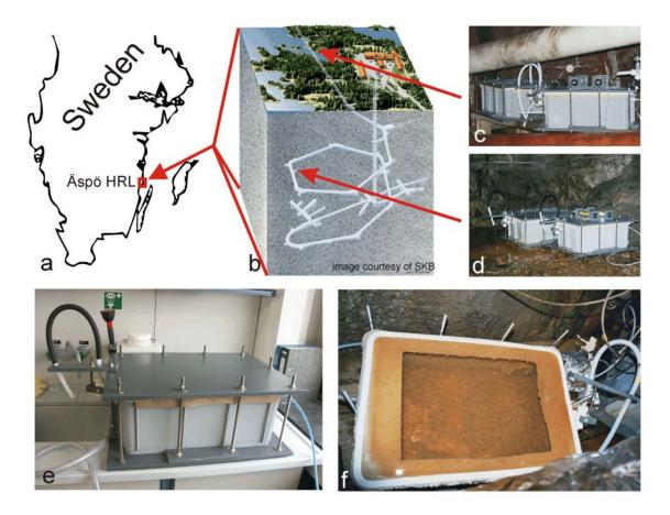
Fig. 5.1 (a) Location of the Äspö Hard Rock Laboratory (HRL); (b) 3D sketch of the HRL tunnel system beneath the island of Äspö; arrows indicate the location of the flow reactor experiments at (c) site 1327B and (d) site 2156B; (e) flow reactor, as used in this study, prior to installation; (f) flow reactor after opening, showing mineralized microbial mat development after two months.
