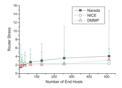
Figure 4.17: Comparison of Router Stress.
