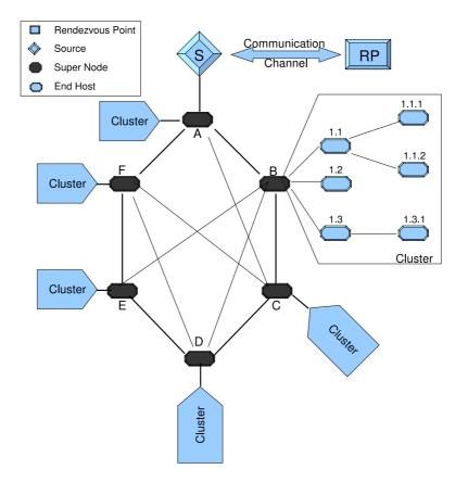
Figure 3.3: Example of DMMP Overlay Hierarchy.
