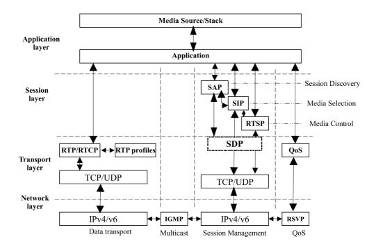
Figure 2.8: Protocol Stacks for Video Streaming
