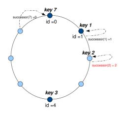
Figure 2.7: Example of Node Joining in Chord.
