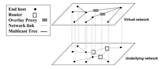
Figure 2.4: High Level Overview of Overlay Multicast.
