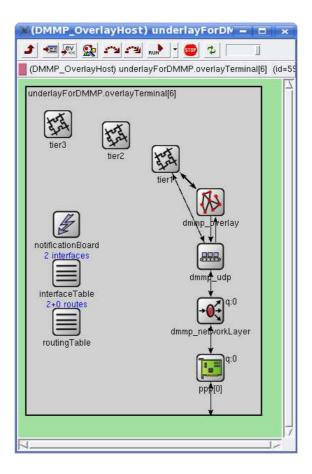
Figure 4.9: The Implemented Protocol Stack of DMMP-aware End Host.
