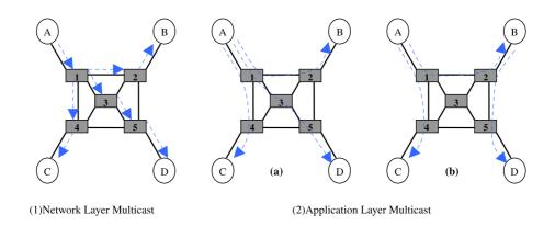
Figure 4.7: Examples of Application Layer Multicast and Network Layer Multicast.
