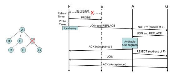
Figure 4.6: Example of Message Flows During Failures.
