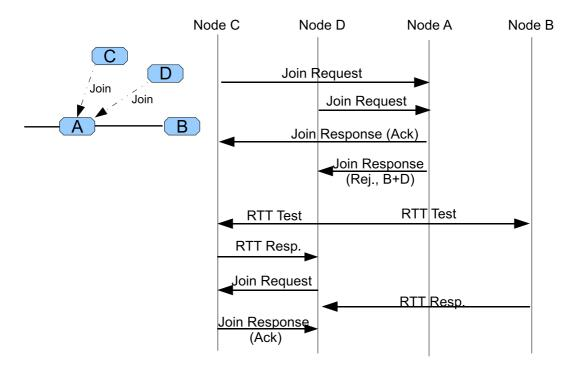
Figure 3.5: Example of DMMP-aware Joining Algorithm.
