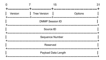
Figure 3.4: DMMP Packet Header Format.
