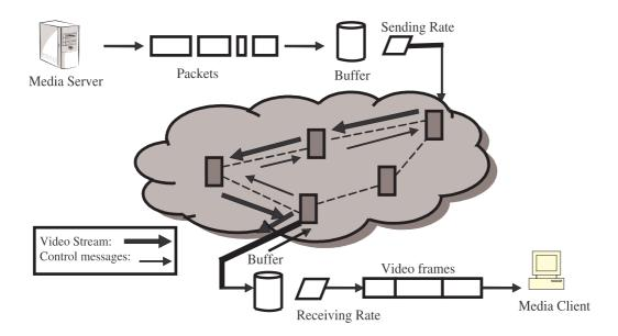
Figure 1.1: Basic Architecture for Video Streaming over the Internet.
