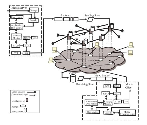
Figure 2.9: Overlay Multicast-based Media Distribution Architecture with Proxy Caching.
