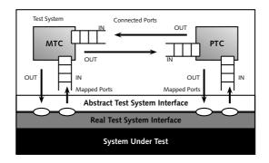
Figure 2.7.: Conceptual view of a typical TTCN-3 test configuration
