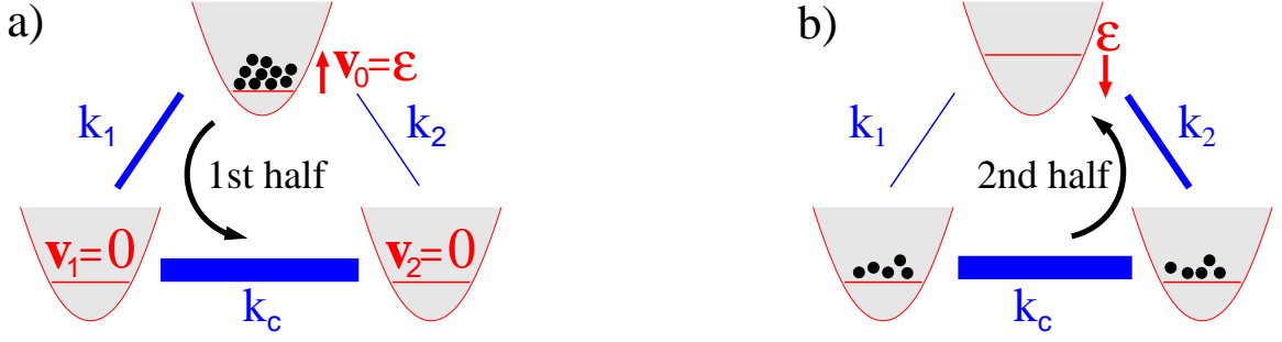
Figure 6.1.: Illustration of the model system. Initially, all particles are located on the upper site ( i = 0 ) which represents the “shuttle”. In the first half of the cycle (a) the on-site potential v_0 = \epsilon is raised adiabatically slow from a very negative initial value and the particles are transported via the k_1 bond to the “canal” which is represented by the strongly coupled canal sites ( i = 1, 2 ). In the second half of the cycle (b) the bias in the coupling is inverted and the particles are transported back from the canal to the shuttle via the k_2 bond.
