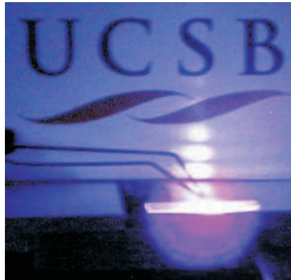
Figure 2.17: Far-field pattern of the world's first non-polar GaN blue-violet laser diode. The bright spots illustrate clear lasing modes (from UCSB Solid State Lighting and Display Center).
