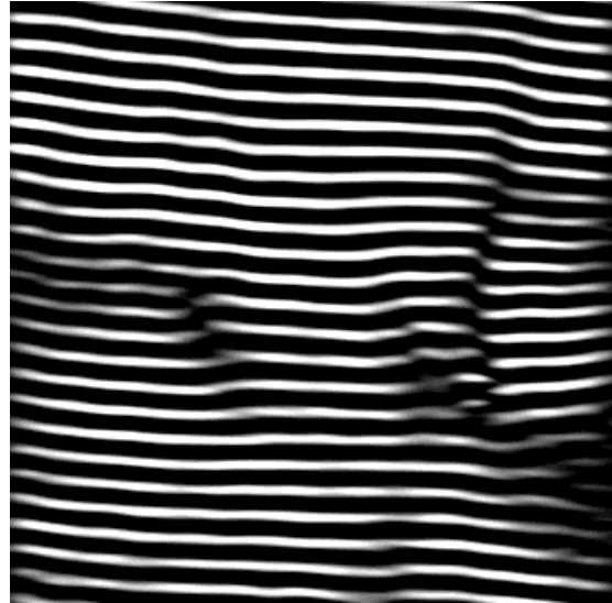
Figure 4.16: Fourier filtered transverse rolls after removing the forced mode \vec{q}_f . The image is the same as in Fig. 4.15.
