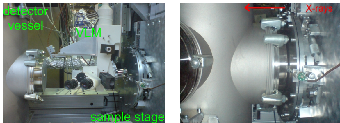
Fig. 4.7: Photographs of the STXM object stage between two vacuum vessels with insertable visible light microscope. Left: Photograph of the STXM object stage when the CCD vacuum vessel (left) is moved back from the zone plate vacuum vessel (right) and the visible light microscope is inserted. Right: Photograph of the object stage when the CCD vacuum vessel is close to the zone plate vacuum vessel, resulting in an air gap of only a few hundred micrometres for soft X-ray imaging. The green board of the stepper motor for stereo experiments is visible.
