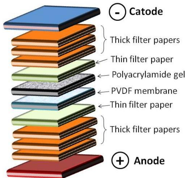
Fig.2. 2 Assembly of a horizontal electroblotting apparatus.
