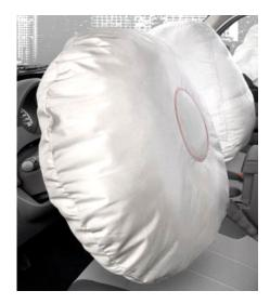
Figure 6.1.: Wrinkles in an inflated airbag.
