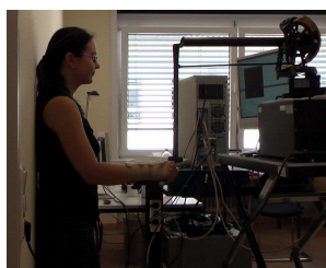
Figure 2.2: Subject standing in front of the manipulandum. The exact position is well-defined by markers on the walls and on the floor. Her back is supported by a wall to prevent swaying. She holds the handle of the manipulandum. The wrist is fixated. Visual feedback for hand positioning is provided on a computer screen.
