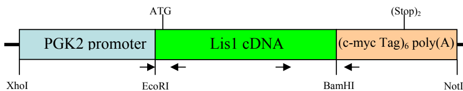
Figure 3.42: Schematic drawing of the PGK2 construct used to generate transgenic mice which overexpress Lis1 gene under control of human PGK2 promoter. A 1377 bp fragment of Lis1 cDNA (containing ATG codon) was cloned into EcoRI and BamHI restriction sites of vector clone 442 (pBluescript II SK (-) with 1.4 kb PGK2 promoter). Next, a 410 bp fragment of (c-mycTag) 6 (containing two stop codons) followed by SV40 poly(A) signal was cloned into BamHI and NotI restriction sites. The black arrows correspond to primers used for genotyping and for RT-PCR analysis.
