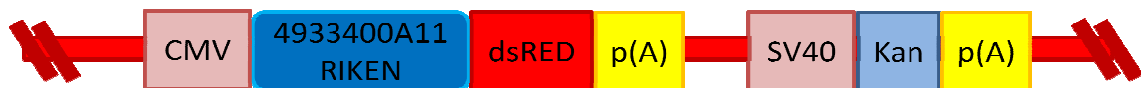
Figure 46. Schematic representation of 4933400A11RikdsRED fusion construct. CMV - CMV IE promoter (human cytomegalovirus immediate early promoter), 4933400A11RIKEN - complete ORF of tested gene, dsRED – dsRed-monomer domain, p(A) – polyadenylation signal, SV40 – SV40 early promoter, Kan – kanamycin resistant cassette.
