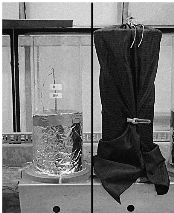
Fig. 3.1: Illustration of the soil columns planted with tree saplings of either species. The measuring modus under maintenance of photosynthesis ( PS = 1 ) is shown to the left, and under complete dark conditions to the right ( PS = 0 ).
