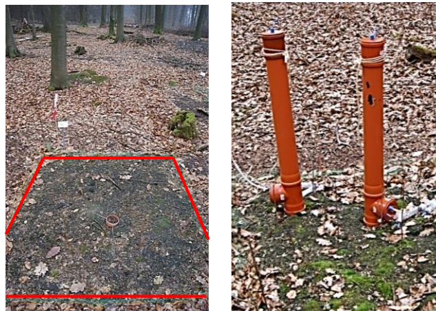
Fig. 5.7: Two plot examples. To the left: the red line shows the rectangular dimension of the plot (180 x 120 cm) and the PVC-collar in its center. To the right: closed PVC-tubes with access ports for gas sampling on the top and devices for maintenance of pressure balance at the bottom.
