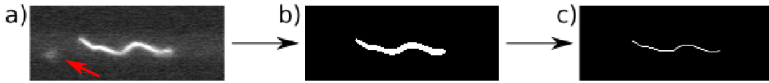
Figure 6.5: Image processing steps a) Original fluorescence microscopy image. Red arrow indicates a fluorescent artifact not connected to the filament. b) After application of a thresholding algorithm and removal of artifacts we obtain a binary image of the recorded fluorescence. c) A one pixel line is calculated by means of a thinning algorithm.
