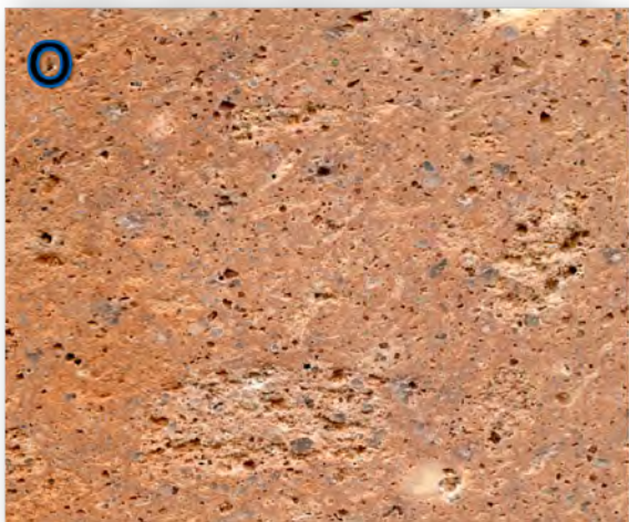
Figure 156: Tuff rocks from Zacatecas. K, M and O, Macroscopic fabric in hand specimen (all samples are a 6.5 cm in length). L, N and P, Thin section of the tuff rocks from Zacatecas (all microphotographs are 5 mm in length and taken with a 5X objective and parallel nicols).
