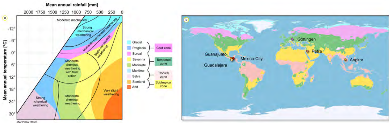
Figure 12: a) Weathering model after Peltier (1950) and b) the locations of the case studies within the different climatic zones.
