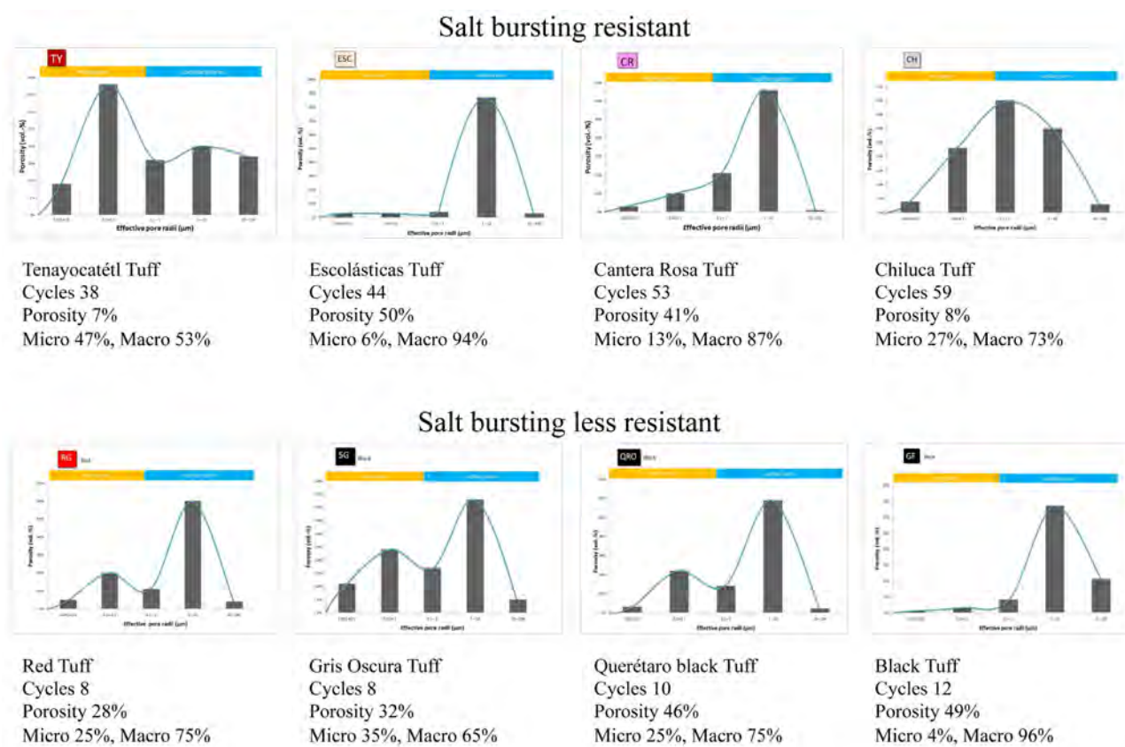
Figure 170: Comparison of the different pore radii distributions between the four resistant (above) and the non-resistant tuffs (below) against salt bursting.
