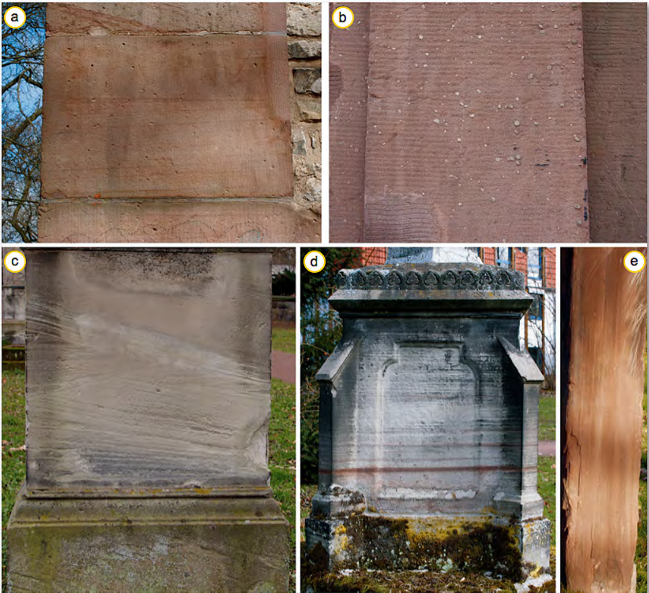
Figure 90: Characteristic sandstone materials of the Bartholomew Cemetery in Goettingen: a) coarsely bedded red sandstone, b) massive red sandstone with white nodules, c) massive gray sandstone with cross-bedding, d) finely bedded sandstone with red-gray interbedded strata and e) finely bedded red sandstone.
