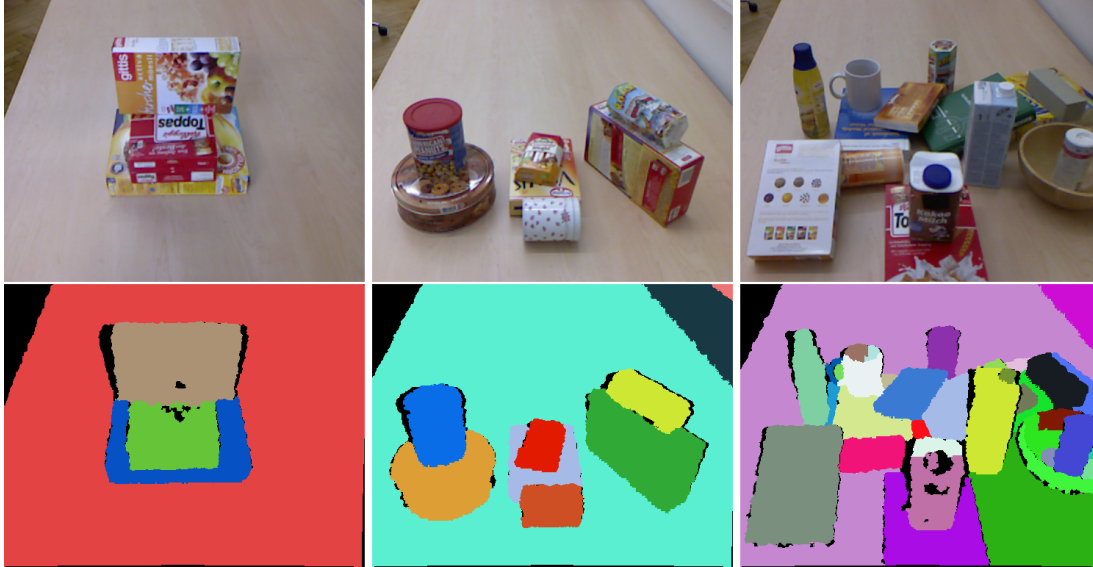
Figure 3.6.6: Example results for the OSD dataset. Points beyond a distance of 2m were cropped for visualization. Parameters: R_{\text{voxel}} = 0.005 , R_{\text{seed}} = 0.02 , \beta_{\text{Thresh}} = 10^\circ .
