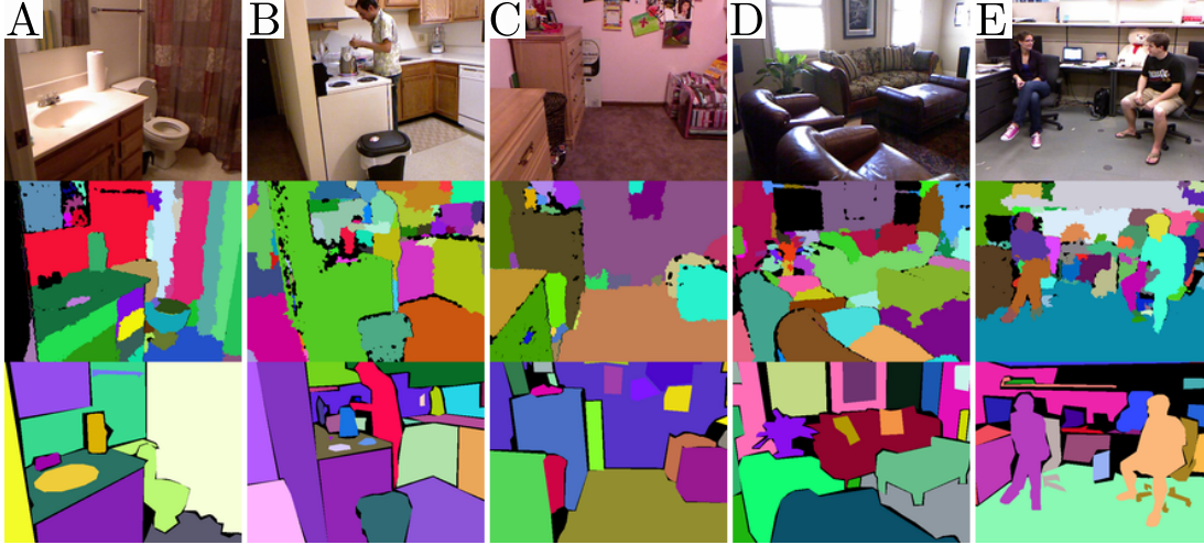
Figure 3.6.1: Example results for scenes from the NYU dataset using unsmoothed depth. Black areas indicate missing depth. Top row: rgb images. Mid. row: segmentation result. Bottom row: ground truth. Parameters A-C: R_{voxel} = 0.0075 , R_{seed} = 0.03 and \beta_{Thresh} = 8^\circ . Parameters D-E: R_{voxel} = 0.01 , R_{seed} = 0.04 and \beta_{Thresh} = 10^\circ (identical to quantitative results, see Tab. 3.6.2).
