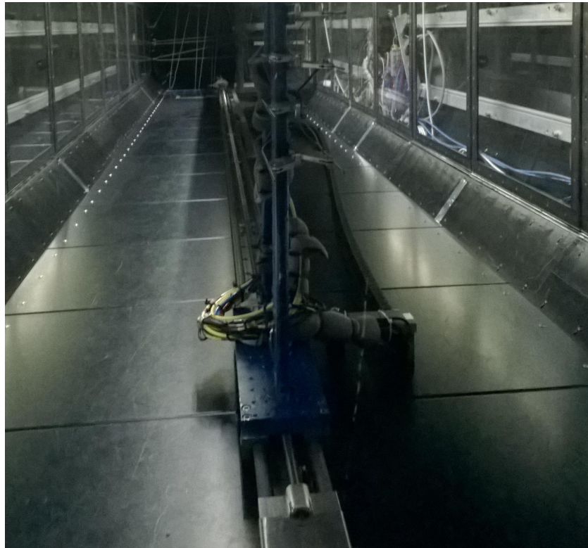
Figure 2.15: Downstream view on the probes and the linear traverse. The traverse is positioned at the nearest position to the grid.
