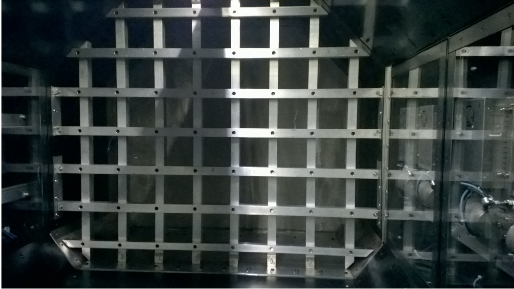
Figure 2.4: Photograph of the-turbulence generating grid, viewing upstream.
