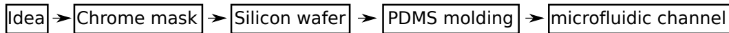
Figure 3.1: Basic idea of soft lithography. After the idea and the concept, using a CAD program a chrome mask will be created. This chrome mask is used to produce a silicon wafer which is the negative image of the PDMS stamp. The PDMS mold is used to built the microfluidic channel.
