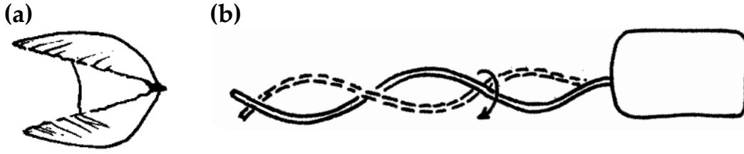
Fig. 2.1: (a) Schematic illustration of a scallop and (b) of a bacterium moving by helical rotation of a flagellum as drawn by Purcell [21]. The scallop will not move at low Reynolds numbers, while the non-reciprocal propulsion in the case of (b) will result in a net-movement of the bacterium.
