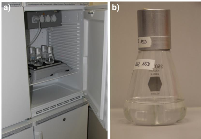
**Figure 1.7 – Experimental setup of time-series experiments** a) Experiments were run in thermostatic cabinets 4 different temperatures and 4 replicates per temperature. b) 250 ml Erlenmeyer borosilicat glass flasks closed with aluminium caps with bottom baffles to increase turbulence and promote gas exchange.
