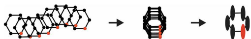
Figure 146: The basic cell approach neglecting the satellite reflections leads to an averaging of the content and large displacement parameters and unusual bond length. Graphics were taken from [150].
