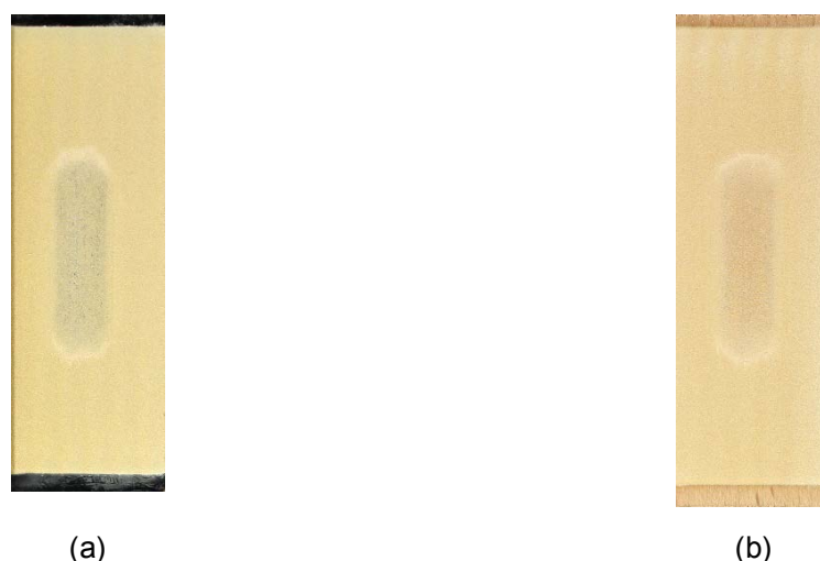
Figure 2: PMMA/ATH + PF coating after 1000 cycles on glass (Fig. 2(a)) and wood (Fig. 2(b)).
