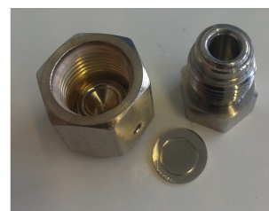
Figure 2.42: About 1 cm 3 hollow screw setup for stability tests of Co containing precursor.
