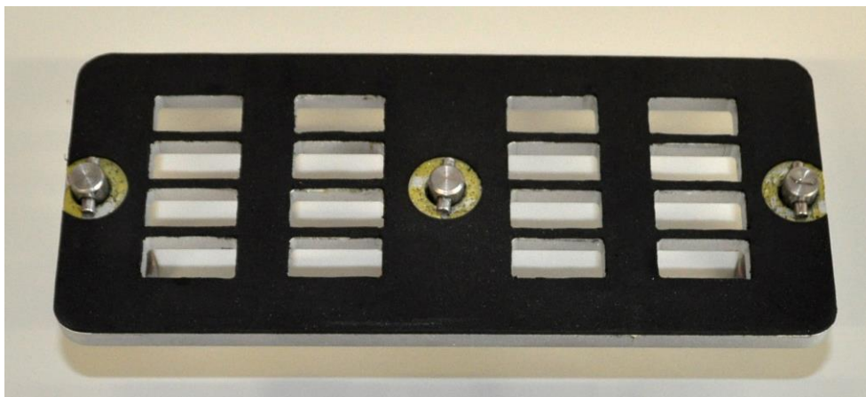
Figure 2–7: Rubber cover of the poxvirus microarray chamber’s lid depicted from below.
