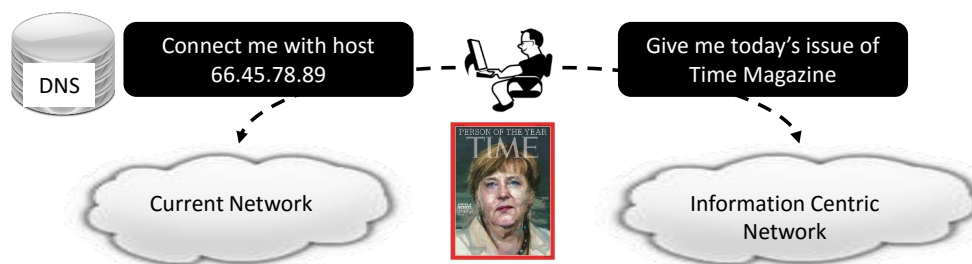
Figure 1.1: An example depicting the difference between IP and ICN at a high level
