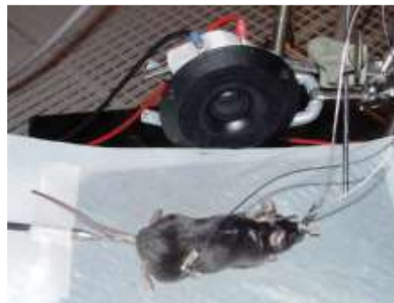
Figure 7. Mouse preparation for the ABR recording. Anesthetized mouse with needle electrodes, inserted subcutaneously. JBL 2402 loudspeaker placed near the left ear (Photo provided by Nicola Strenzke)
