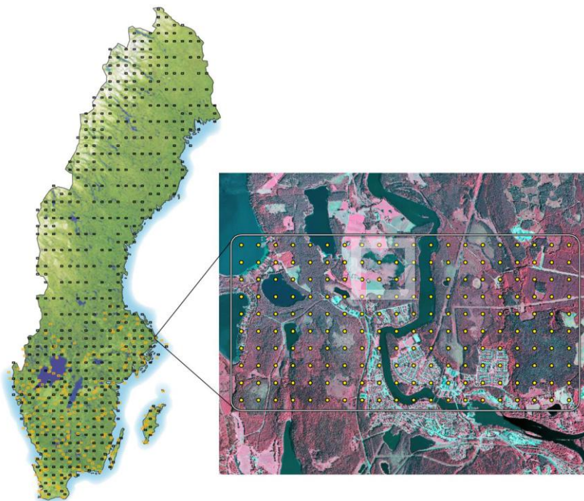
Figure 11. MOTH 2-phase sampling for stratification with aerial infrared imagery and overlap with NFI sample plots. The map shows the 565 stratified sample units. Infrared images are acquired for every unit and a 5 km x 2.5 km point-grid is superimposed. The 200 points are interpreted and visually classified. 12 of the of the 2000 MOTH grid points overlap with 12 NILS field sample plots (highlighted by the white shaded frame). In the second phase, a percentage of MOTH points in every class is randomly selected for field visits. (amended after: Gardfjell, 2014; Adler, 2014)
