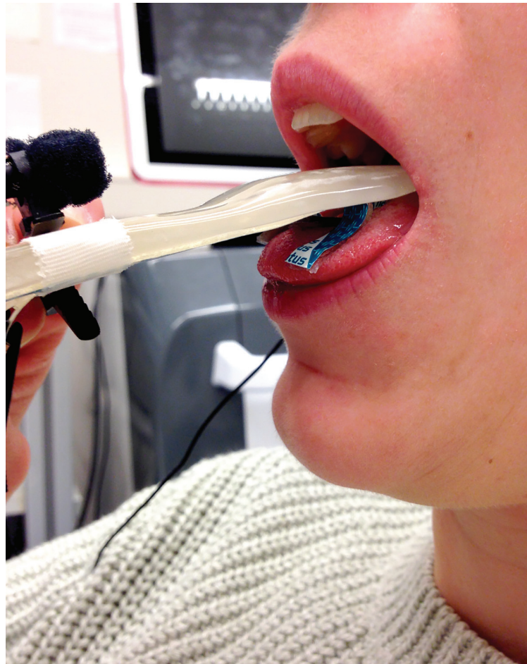
Fig 1. Tongue setup. The electrodes are secured to the underside of the mouthpiece and rest on the tongue. The microphone is also attached to the mouthpiece, visible on the left.
