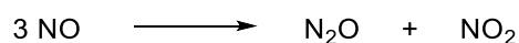
Scheme 37. Simple disproportionation of nitric oxide to give nitrous oxide and nitrogen dioxide.
