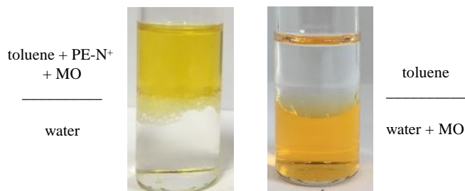
Figure 5-5. Resulting two-phase system of PE-N + in toluene, MO and water (left) and toluene, MO and water (right) after mixing at 90 °C.
