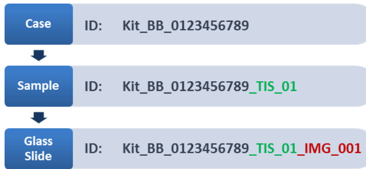
Figure 4.5. Identification of pathology information in STARLIMS. A Case ID is represented with a 17-digit sequence of numbers and letters separated by an underscore. The Sample ID consists of Case ID and a suffix “_TIS_” along with an auto incremented 2-digit number (suffix is written in green). A Glass ID is represented with the Sample ID and the suffix highlighted in red.
