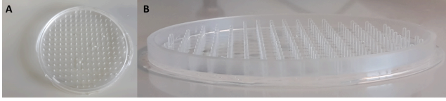
Fig.S 1. (A) Top view and (B) side view of the PDMS block with a quadratic arrangement of the pillars that fits to a normal 100 mm plastic Petri dish. The pillars are 1 mm thick, 3 mm high and are spaced 5 mm away from each other.
