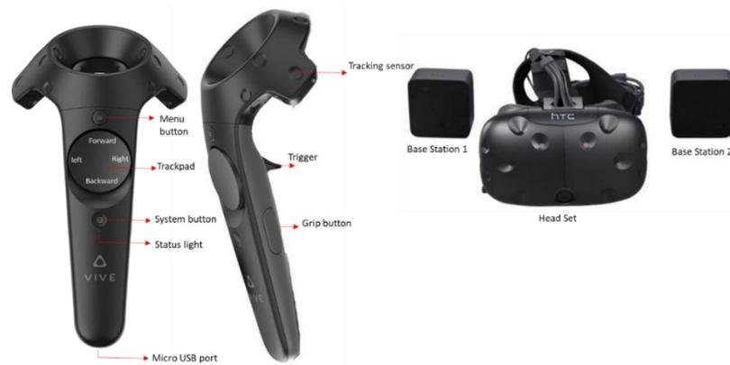
**Figure 4.6:** HTC VIVE headset, base stations and two hand controller showing the required functionality of its buttons.
