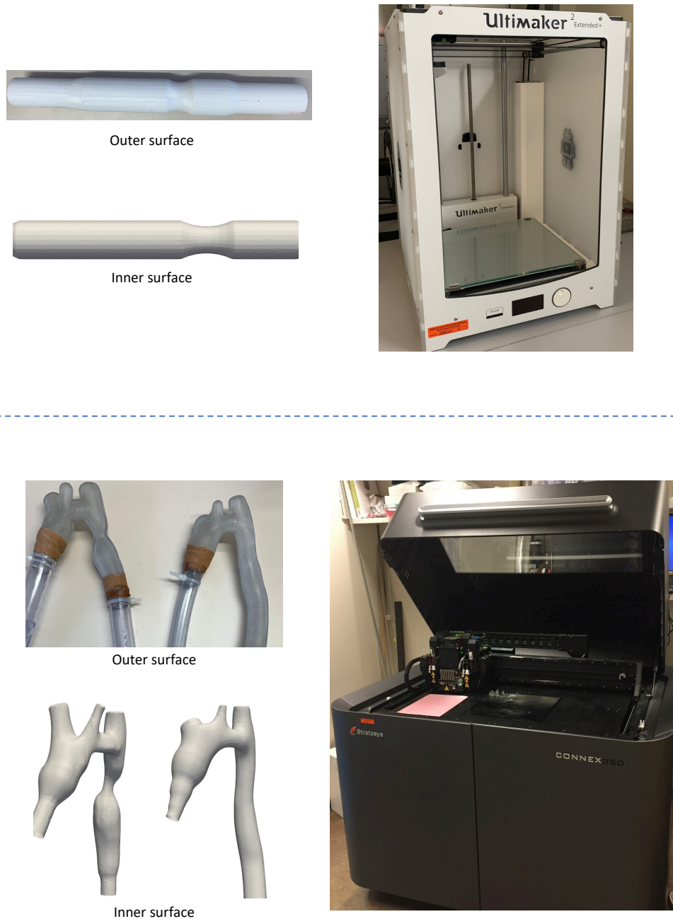
FIGURE 2.4: 3D printed phantoms and the corresponding printers used. Top, a straight pipe with stenosis; bottom, two aortic geometries. For each phantom, the inner surface was created based on specified dimensions or image segmentation, while the outer surface was obtained by extruding the inner surface to a given thickness for the purpose of 3D printing. More details of the phantoms are provided in Chapters 3 and 4.
