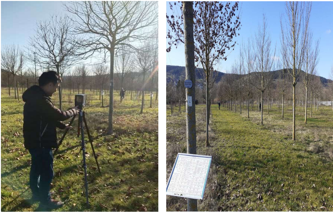
Figure 1.2 A tripod-mounted Faro Focus 3D TLS (Faro Focus M70 Terrestrial Laser Scanner) that is placed 1.3 meters above the ground at the Stutel-Arboretum.
