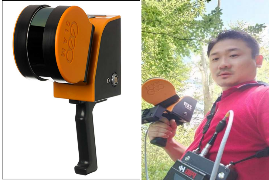
Figure 1.1 Hand-held mobile scanning device (ZEB HORIZON, GeoSLAM, 2019) used in this study.
