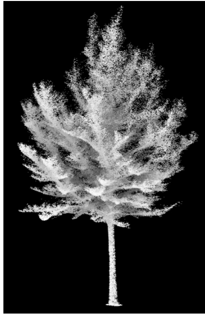
Figure 3.3 Exemplary cleaned and filtered 3D point cloud of an Elm tree ( Ulmus ) obtained from mobile laser scanning
