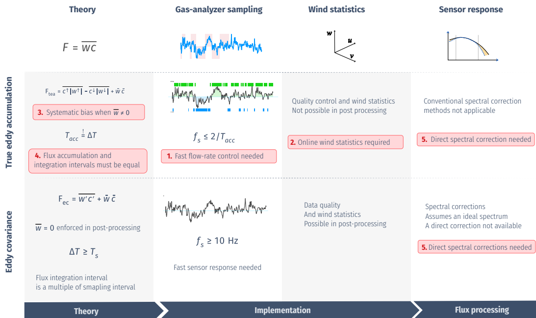
Figure 1.3: Conceptual figure showing the main true eddy accumulation challenges addressed in this thesis categorized by four distinct categories. The challenges are numbered by the order they appear in the thesis. A comparison with the eddy covariance method for each category is provided as a reference.
