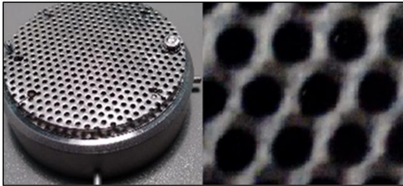
Figure 3.3: Sputter holder with the mask used to deposit the Pd dot pattern onto the glass substrate. Hole sizes of 1 mm (left-hand side) result in deposited dot pattern of 1.4 mm (right-hand side).
