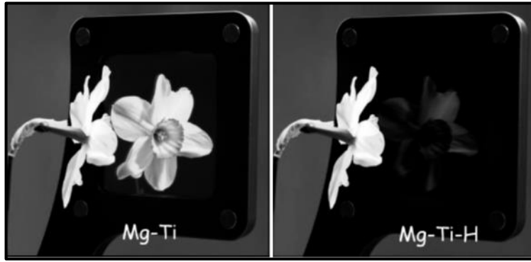
Figure 3.6: Mg 0.7 Ti 0.3 thin film in, the metallic (left) and the hydride (right) state during hydrogenation [104]. Reprinted with permission from [104]. copyright 2008 Elsevier.
