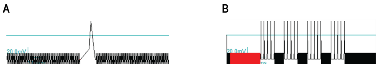
Figure 2. 3 (A) Single voltage ramp imitated by three ramps and (B) four-burst AP-like ramps stimulation.
