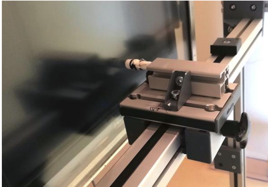
Figure 11: Artificial finger (ArFi). The black handle is manipulated by the monkeys allowing them to slide the artificial finger (white stab) along the touchscreen to perform a swiping task.
