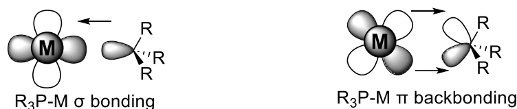
Figure 8. Phosphines are L-type ligands that undergo backbonding with transition metals through d_{\pi}-\sigma^* interaction.
