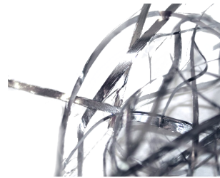
Figure 2.6: Photograph (own work) of a melt spun MG ribbon of \text{Zr}_{65}\text{Cu}_{27.5}\text{Al}_{7.5} .
