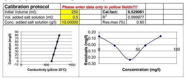
Figure 4.4: Calibration Curve of Auja Spring, Experimental Measurement of Spring discharge, June, (2013)
