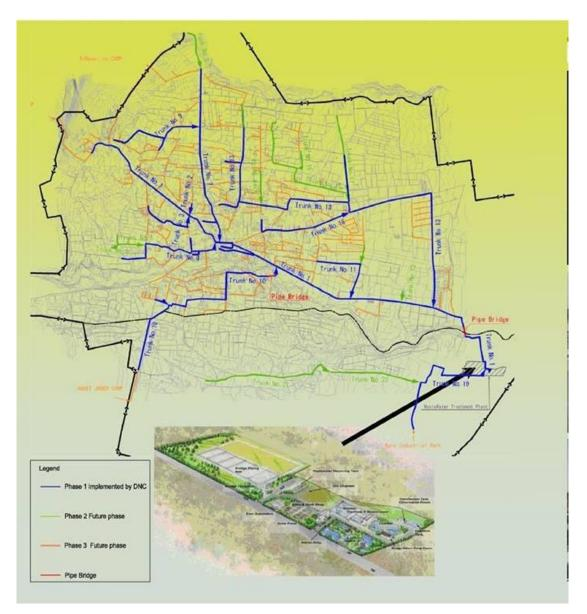
Figure 4.11: JWWTP site location sketch design of JWWTP including sewer pipes of future phases (JICA, PWA, Jericho Municipality (JM), 2014).
