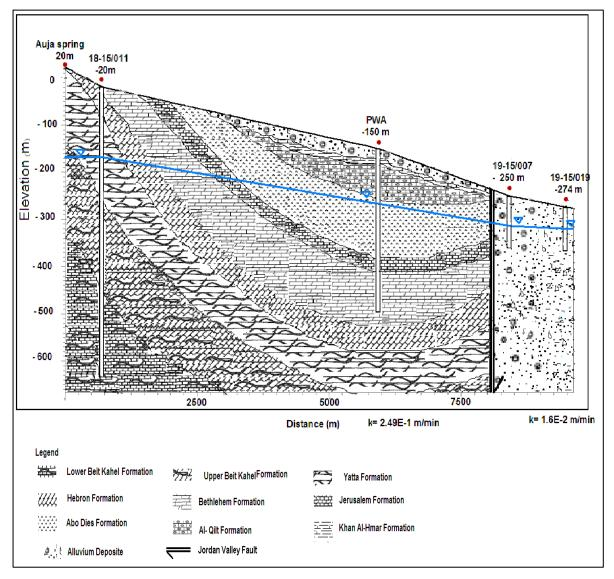
Figure 2.20: Hydrogeological cross section from west to east showing the groundwater table. PWA, Amer Marei, 2013.
