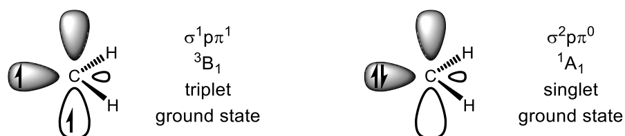
Scheme 11. Schematic illustration of the two appropriate ground states for carbenes using the example of (:CH 2 ). Left: triplet ( \sigma^1 p\pi^1 , ^3B_1 , spin unpaired); right: singlet ( \sigma^2 , ^1A_1 , spin paired). [33,34]
