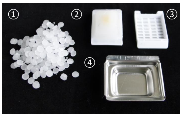
Fig. 9 Material for Paraffin embedding (1) Paraffin pellets (2) cassette with sample embedded in paraffin (3) empty cassette and (4) embedding mould.
