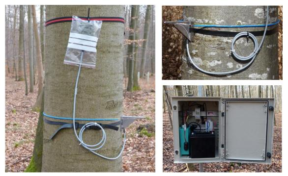
**Fig. 1.2:** Electronic self-acting DC2 circumference dendrometer with Scatter 100 sensor unit (left respectively top right) and Scatter 100 base station (bottom right).
