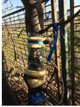
Figure 9: sampling procedure on a tree trunk. The analysed part is wrapped in Nalophan foil, closed with staples and tension belts.
