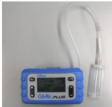
Figure 10: Sampling procedure for beetles, pupae and frass. The samples are stored in the headspace vial while sampling with the pump
