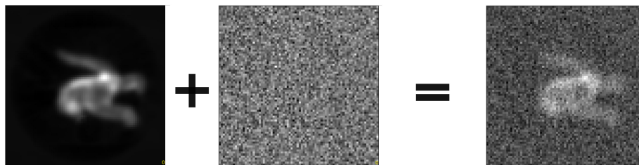
Figure 1.9: Synthetic additive image noise The first summand is a projection image of a simulated 3D density map. The map was noise free so that the projection image contains the predicted (resp. ideal) signal. The second summand is a pure Gaussian distributed noise image simulated in MATLAB. The sum of both images represent the measured signal. It is distorted due to a variety of effects.
